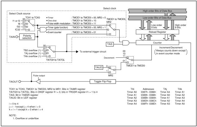
Figure 12.3 Timer A Block Diagram
